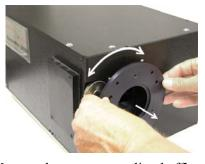
**7.** Mount tube to camera, align baffle with **8.** Gently rotate while inserting. bottom/top of camera, and tighten mounting screws.
